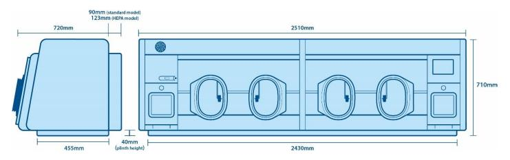
**Important note:** In addition to the dimensions stated above, allow a localised protrusion of 90mm at rear to accommodate condenser bottle, bracket, gas and electrical supplies. If bench mounted, a further minimum clearance of 500mm is required above the unit and a minimum clearance of 500mm at the right-hand side of the unit is required for user/service access.
